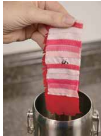
Stained Multifiber from Rotawash Container
