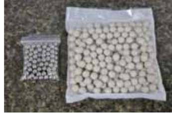
Ball Bearings for Colorfastness Testing
