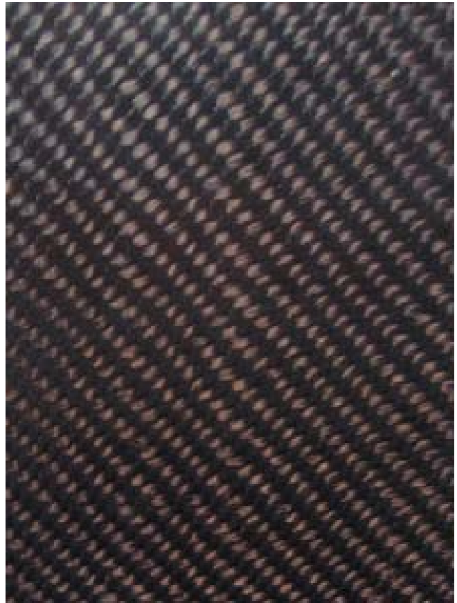
Carbon fiber and polypropylene thread being tested for strength before being made into its final composite of a solid sheet.
