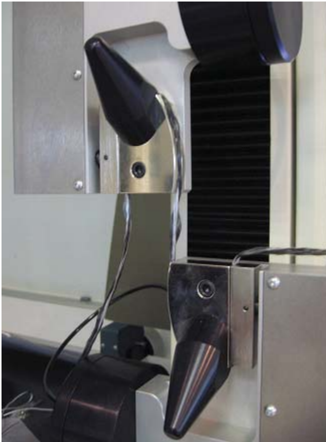
Carbon fiber and polypropylene thread being tested for strength before being made into its final composite of a solid sheet.
