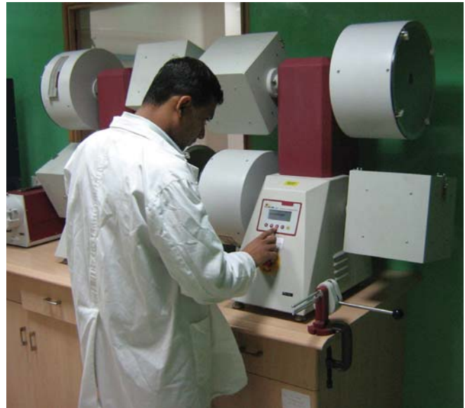
Setting a test on the SDL Atlas ICI Pilling Tester
