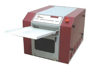
Lint and Trash Analyzer MK2 (Cotton Model). To determine lint, trash and dust content within a sample of cotton fiber up to 100 grams. Also used to determine non-fiber content of synthetic fibers and to open and clean fibers for further testing. The analyzer uses the carding principle with air separation of lint and non-lint content.
